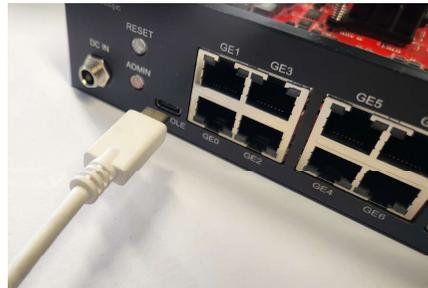
Use a USB-C console cable of your choice to connect the onboard serial console converter.
