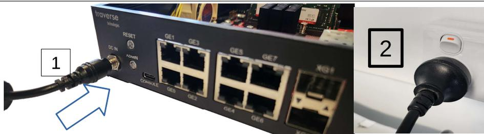
Insert the DC connector into the appliance **first**, then plug in the AC lead. This reduces disruption to other devices when the appliance is powered on.
